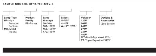
Options (add as suffix) <sup>6</sup> Q=Quartz Restrike (Lamp by others) F1=Single Fuse (120, 277 or 347V) F2=Double Fused (208, 240 or 480V) QM=Quick Mount LL=Lamp Included <sup>6</sup> TR=Tamper Resistant Screws Accessories (order separately) TK=Trunnion Kit VRSD=Tamper-Resistant Screwdriver VRSB=Tamper-Resistant Bit
